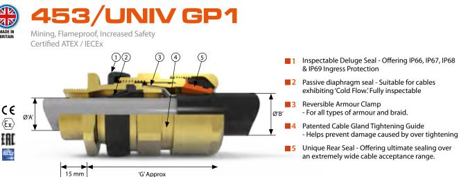
The 453 Universal group I mining Cable Gland is dual certified Exe/Exd, robust and for use with single wire armour 'W', wire braid 'X', steel tape armour 'Z', elastomer and plastic insulated cables. For particular use with cables that exhibit 'Cold Flow' characteristics, with a fully inspectable passive inner diaphragm seal. See technical section for installation rules and regulations
