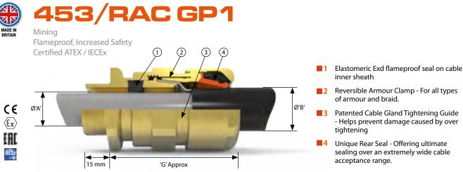
The 453/RAC group I mining Cable Gland is dual certified Exe/Exd, robust and for use with single wire armour 'W', wire braid 'X', steel tape armour 'Z', elastomer and plastic insulated cables The gland provides an elastomeric seal on the cable inner sheath, and a low smoke, zero halogen IP and retention seal onto the cable outer sheath. See technical section for installation rules and regulations
